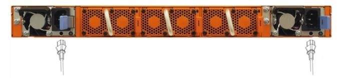
Figure 16: Connecting AC Power on a GigaVUE-TA100
