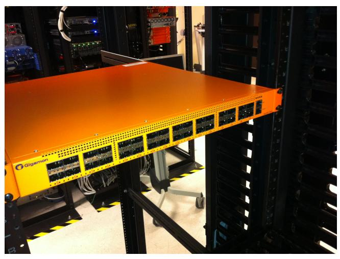
Figure 11: Front View of the Mounted Node to the Four-Post Rack
